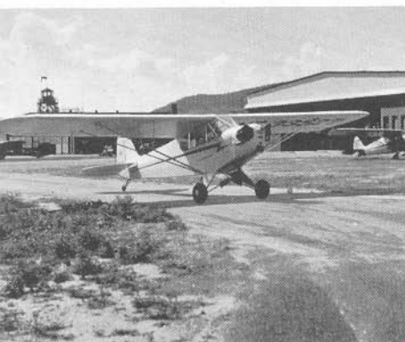
15. Observe the windsock and S-taxi to the runway. Always take off and land INTO the wind. Do not taxi faster than normal walking speed. Look around and ahead constantly for other aircraft.
