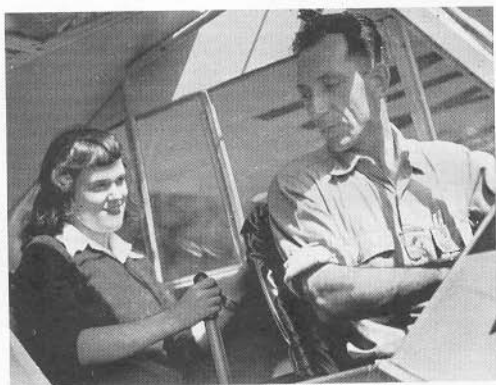
6. Check rudder and stick controls for freedom of movement by moving them in all positions.
