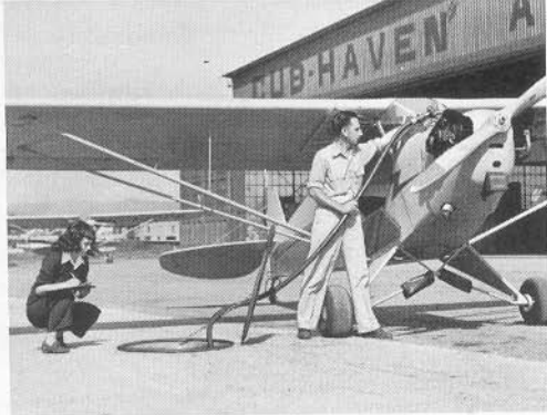
2. Always check the gas by the gauge and by looking into tank. Fill the tank when necessary.
