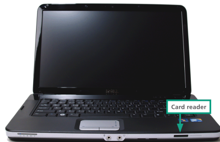
Many digital devices are equipped with a card reader for transferring data to and from solid state memory cards.
