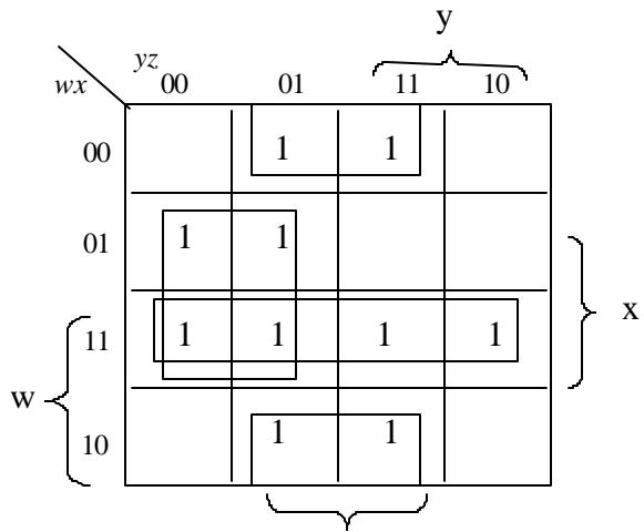
$$\begin{aligned} F &= \Sigma(1, 3, 4, 5, 9, 11, 12, 13, 14, 15) \\ &= wx + xy' + x'z \end{aligned}$$
