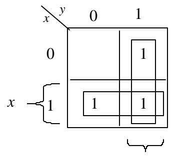
$$\begin{aligned} F &= x + y \\ &= x'y' + xy' + xy \end{aligned}$$
