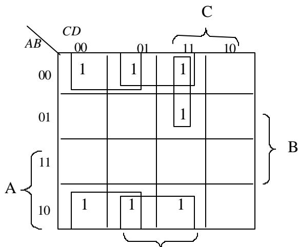
$$\begin{aligned} F &= A'B'C' + B'CD + A'BCD + AB'C' \\ &= B'D + B'C' + A'CD \end{aligned}$$
